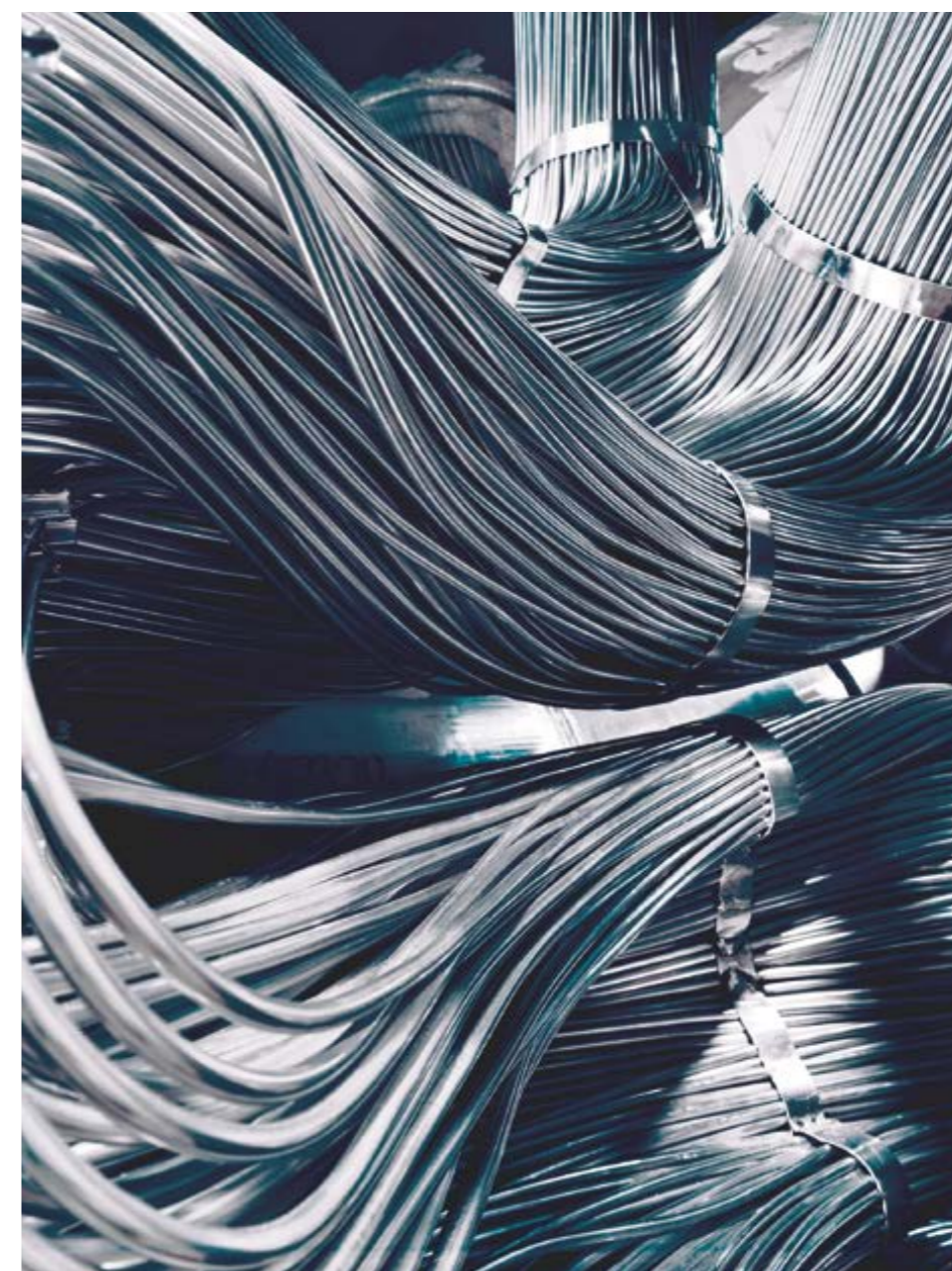
Coil-wound heat exchangers are used across a broad spectrum of cryogenic applications.
