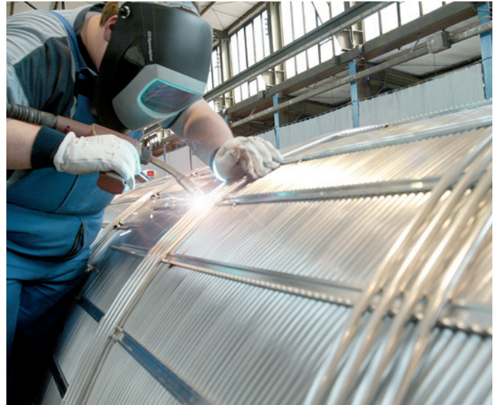
Coil-wound heat exchanger fabrication at the Linde facility in Schalchen, Germany
