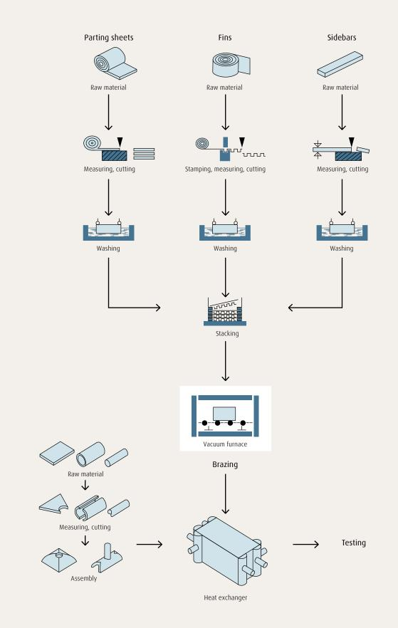
PFHEs are manufactured from raw materials in a multi-step process with all steps rigorously controlled to ensure the highest quality. After the headers and nozzles have been welded to the core, the completed heat exchangers are subjected to non-destructive testing. This includes hydraulic or pneumatic pressure testing and leak testing.
