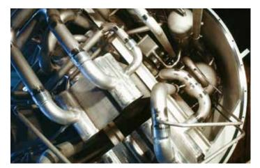
Helium liquefaction unit.
