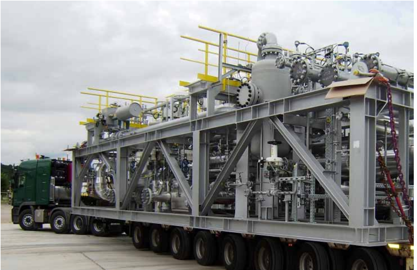
Skid-mounted solution for a purge gas recovery unit, ready for shipment.
